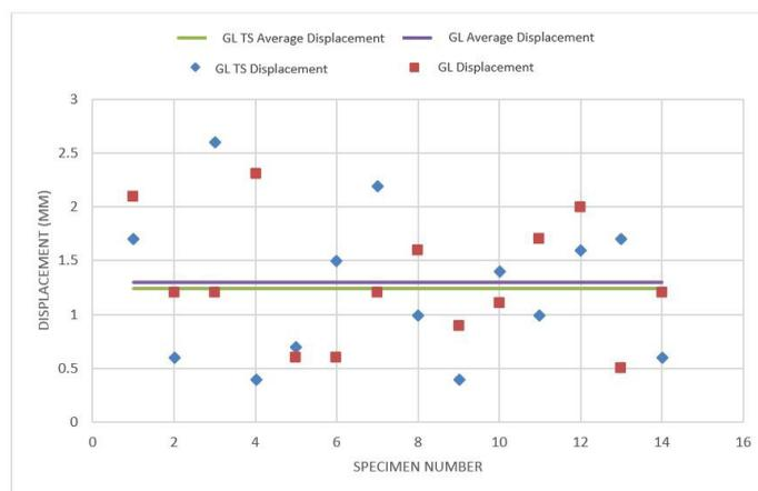
**Figure 3. Average displacement for each GL and GL TS Specimen with group averages.**
