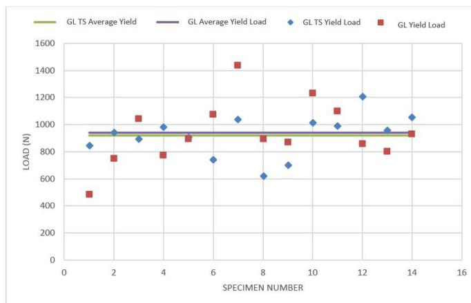
**Figure 2. Yield load for each GL and GL TS Specimen with group averages.**
