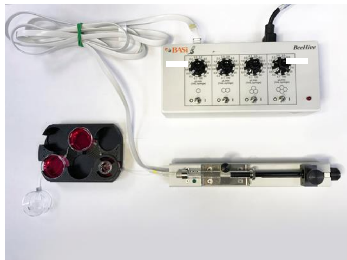
Figure 1. The three compartment HuDMOP™ system routinely used at IONTOX (intestine – liver – kidney) complete with pump. Each cell or tissue type remains in its own optimal media, so the media is not circulated between compartments.
