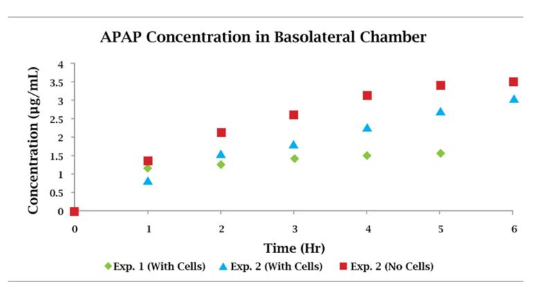
APAP kinetics were measured with (green and blue symbols) and without (red symbol) Caco-2 cells. APAP movement from the apical chamber to the basolateral chamber was slightly slower in the presence of cells.
