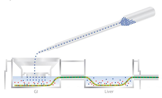
A simple two-compartment organ model was tested by adding a single bolus concentration (200 µM) of Acetaminophen (APAP) to the apical side of the Caco-2 chamber, then periodically measuring APAP concentrations throughout the system. Each simulated-organ compartment was essentially isolated from the other compartments. Movement of drug between organ chambers was solely by the fluidics system.
