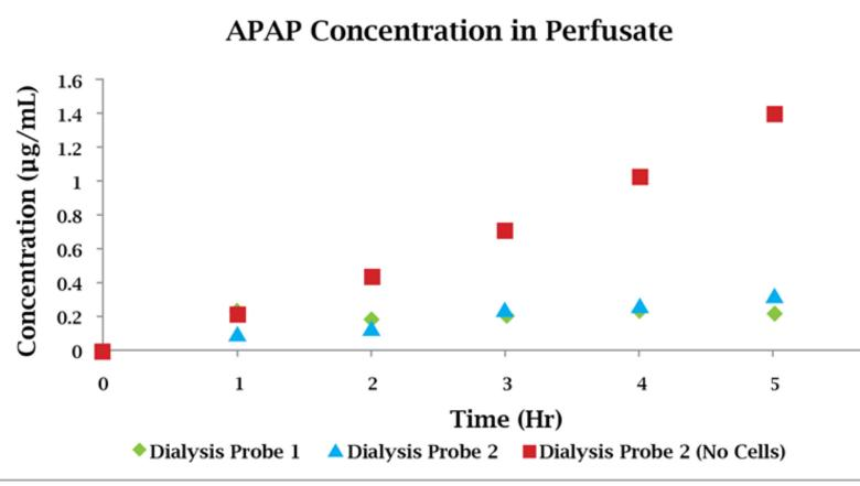
APAP concentration in the fluidics system (perfusate) reached its maximum concentration by 5 hr in the absence of cells (red symbols). In the presence of cells, concentrations in the perfusate were significantly lower (green and blue symbols). This delay in the increase in APAP concentration was most likely due to rapid cellular (HepG2) uptake. Concentrations at each time point were determined from perfusate samples collected over the sample interval.
